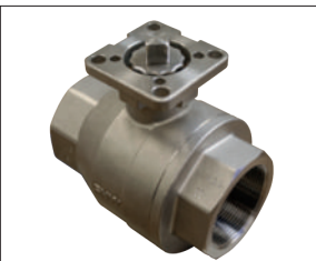
Figure 220AM 2 PC FULL PORT 2000 CWP ISO MOUNT SS BALL VALVE • ISO 5211 MOUNTING PAD • 150 PSI WSP • LIVE LOADED PACKING • INVESTMENT CAST BODY & END CAP • TFM SEATS • FOR DIRECT MOUNT ACTUATION • SIZES 1/4" - 3"
