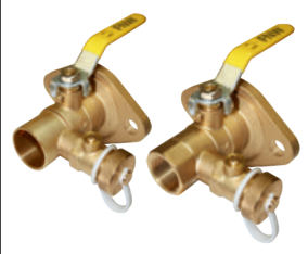
Figure 490D / 495D 2 PC FULL PORT 600 WOG PUMP ISOLATION BALL VALVE w/ ROTATING FLANGE & DRAIN • INTEGRAL ROTATING PUMP FLANGE CONNECTION & ON/OFF DRAIN • FNPT END (490D), SWEAT END (495D) • INCLUDES T-HANDLE, GASKET & BOLTS • SIZES 3/4" - 1 1/4"
