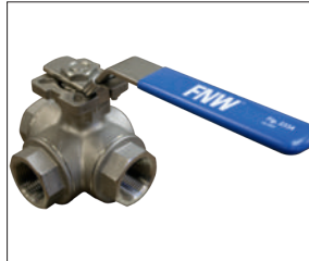
Figure 233A 3-WAY DIVERTER 1000 CWP STAINLESS STEEL BALL VALVE • STANDARD PORT • 150 PSI WSP • RTFE SEATS • SS LOCKING HANDLE • BLOW-OUT PROOF STEM • ISO 5211 MOUNTING PAD • SIZES 1/2" - 2"
