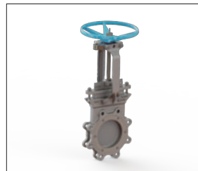
Figure 2020 HIGH PERFORMANCE KNIFE GATE VALVE • CAST SS BODY/YOKE/FOLLOWER • O-RING ENERGIZED REINFORCED TEFLON RESILIENT SEATS • BI-DIRECTIONAL SHUTOFF • STAINLESS NEEDLE BEARING FOR REDUCED HW TORQUE • ELASTOMER QUAD SEAL IN PACKING • SIZES 2" - 24"
