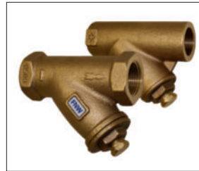
Figure 509 / 510 BRONZE Y-STRAINER • 250 WOG, 150 PSI STEAM (509) • 400 WOG, 250 PSI STEAM (510) • 510 IS 400 WOG, 250 PSI STEAM • CAST BRONZE BODY • 20 MESH STAINLESS STEEL SCREEN • BLOW-OFF PLUG INCLUDED • SIZES 3/8" - 2" (509); SIZES 1/2" - 2" (510)
