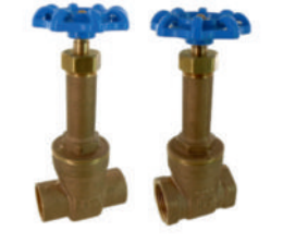
Figure 1221 / 1222 RS 125# BRONZE GATE VALVE • 200 CWP • 125 PSI STEAM RATED (1221 ONLY) • SOLID WEDGE DISC • FNPT (1221) & SWEAT (1222) ENDS • BACK SEAT DESIGN • CONFORMS TO MSS SP-80 • SIZES 1/2" - 3"
