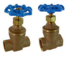
Figure 1211 / 1212 NRS 125# BRONZE GATE VALVE • 200 CWP • 125 PSI STEAM RATED (1211 ONLY) • SOLID WEDGE DISC • FNPT (1211) & SWEAT (1212) ENDS • BACK SEAT DESIGN • CONFORMS TO MSS SP-80 • SIZES 1/4" - 3" (1211); SIZES 1/2" - 3" (1212)
