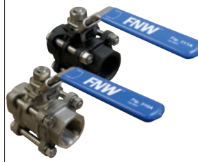
Figure 310A - SSxSS Figure 311A - CSxSS 3 PC FULL PORT 1000 CWP BALL VALVE • INVESTMENT CAST BODY & END CAPS • 150 PSI WSP • NPT ENDS (OPTIONAL SOCKET WELD) • SS LOCKING HANDLE • RTFE SEAT • SIZES 1/4" - 3"
