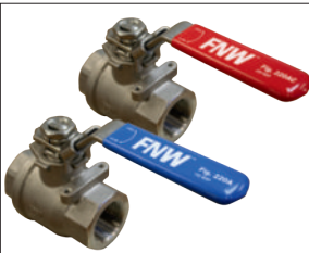
Figure 220A / 220AC - SSxSS Figure 221A / 221AC - CSxSS 2 PC FULL PORT 2000 CWP BALL VALVE • INVESTMENT CAST BODY & END CAP • 150 PSI WSP (220A/221A) • 250 PSI WSP (220AC/221AC) • SS LOCKING HANDLE • TFM SEATS • SIZES 1/4" - 3"
