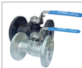
Figure 500B - SSxSS Figure 501B - CSxSS 1 PC STANDARD PORT 150# FLANGED BALL VALVE • INVESTMENT CAST BODY • ANTI-STATIC DESIGN • TFM SEATS • ISO MOUNTING PAD • SIZES 2" - 6" Figure 500C & 501C • Fire Safe
