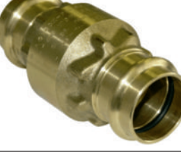
Figure 431 200 PSI PRESS CONNECTION BRASS IN-LINE CHECK VALVE FOR WATER • HIGH CAPACITY DESIGN • LOW 1/2 PSI CRACKING PRESSURE • SOFT SEAT FOR TIGHT SHUTOFF • NSF-61 APPROVED • FORGED BODY & END CAP • SIZES 1/2" - 2"
