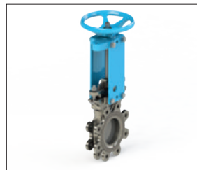
Figure 6701 CAST SS KNIFE GATE VALVE, METAL SEATED • CAST SS BODY AND FOLLOWER • INTEGRAL METAL SEAT • CARBON STEEL & IRON TOPWORKS • UNI-DIRECTIONAL SHUTOFF • DESIGNED FOR HEAVY MEDIA • NON-CLOGGING STEP SEAT DESIGN • SIZES 3" - 30"
