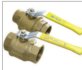
Figure 420 / 421 2 PC FULL PORT 600 WOG BRASS BALL VALVE
