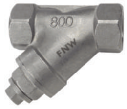
Figure 14B-YSS THREADED SS 800 PSI CWP Y-STRAINER • SS 20 MESH SCREEN • VITON® O-RING SEAL • SIZES 1/2" - 2"
