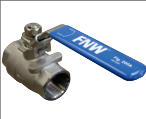
Figure 200A 2 PC FULL PORT 1000 CWP STAINLESS STEEL BALL VALVE • INVESTMENT CAST BODY & END CAP • 150 PSI WSP • SS LOCKING HANDLE • RTFE SEATS • BLOW-OUT PROOF STEM • SIZES 1/4" - 2"
