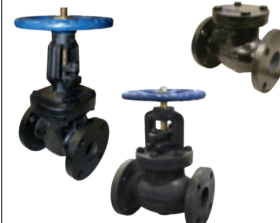
Figure 651A / 661 / 671A 125# IRON BODY, BRONZE MOUNTED VALVE • IBBM GATE (651A), GLOBE (661), & CHECK (671A) VALVES • 125 PSI SWP (SATURATED TO 353°F) • DESIGN AND TESTED TO: • GATES: MSS SP-70 • GLOBES: MSS SP-85 • CHECKS: MSS SP-71
