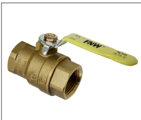
Figure 410A 2 PC FULL PORT 600 WOG BRASS BALL VALVE
