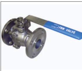
Figure 660A 2 PC FULL PORT 150# FLANGED ECONOMY BALL VALVE • INVESTMENT CAST BODY • ANTI-STATIC DESIGN • RTFE SEATS • ISO MOUNTING PAD • SIZES 2" - 6"
