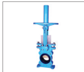
Figure 60R KNIFE GATE VALVE FOR ABRASIVE APPLICATIONS • CAST CS BODY/YOKE/FOLLOWER • RESILIENT SEAT • POP-OUT SLEEVE-LINED • BI-DIRECTIONAL SHUTOFF • UP TO 100 PSI CWP • SIZES 3" - 30"
