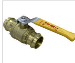
Figure 435 125 PSI PRESS CONNECTION BRASS BALL VALVE FOR GAS SERVICE
