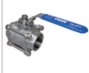
Figure 360A 3 PC FULL PORT STAINLESS STEEL BALL VALVE 1000 WOG • 150 PSI/WSP • WORKING TEMP: -4°F - 392°F • INVESTMENT CAST BODY • BLOW OUT PROOF STEM • ISO 5211 MOUNTING PAD • STAINLESS STEEL HANDLE • LOCKING LEVER • SIZES 1/4" - 3"
