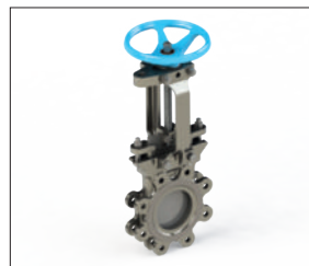
Figure 6500 CAST SS KNIFE GATE VALVE, METAL SEATED • CAST SS BODY/YOKE/FOLLOWER • INTEGRAL METAL SEAT • UNI-DIRECTIONAL SHUTOFF • DESIGNED FOR HEAVY MEDIA • GATE EDGE RADIUS • ANTI-EXTRUSION RING IN PACKING • ELASTOMER QUAD SEAL IN PACKING • SIZES 2" - 24"
