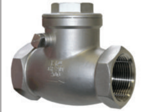
Figure 16B-200 THREADED SS 200 WOG SWING CHECK VALVE • STAINLESS STEEL TRIM • PTFE SEALS • SIZES 1/4" - 2"
