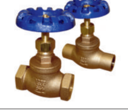
Figure 1231 / 1232 125# BRONZE GLOBE VALVE • 200 WOG • 125 PSI STEAM RATED (1231 ONLY) • RESILIENT SEAT DISC • FNPT (1231) & SWEAT (1232) ENDS • CONFORMS TO MSS SP-80 • SIZES 1/4" - 3" (1231); SIZES 1/2" - 2" (1232)
