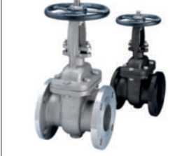
Figure 451A / 452A - SS Figure 551 / 552 - CS FLANGED OS&Y WEDGE GATE VALVE • 150# FLANGES (451A/551) • 300# FLANGES (452A/552) • API 600 (CS), API 603 (SS) • INVESTMENT CAST TO 8" (SS ONLY) • FLEX WEDGE DESIGN FOR POSITIVE SHUTOFF
