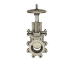
Figure 62B LINED KNIFE GATE VALVE, RESILIENT SEATED • CAST DI BODY/SS LINED • POSITIVE SHUTOFF RESILIENT SEAT • SS WETTED PARTS • UNI-DIRECTIONAL SHUTOFF • ECONOMY VALVE FOR MANY APPLICATIONS • SIZES 3" - 24"
