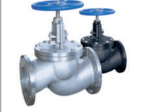
Figure 461A / 462A - SS Figure 561 / 562 - CS FLANGED GLOBE VALVE • 150# FLANGES (461A/561) • 300# FLANGES (462A/562) • API 600 (CS), API 603 (SS) • INVESTMENT CAST TO 8" (SS ONLY) • MODIFIED PLUG TYPE DISC FOR HAND OPERATED THROTTLING
