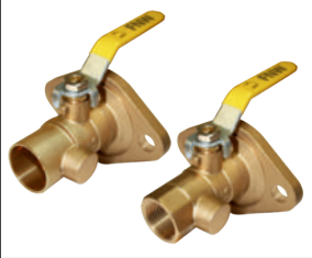
Figure 490 / 495 2 PC FULL PORT 600 WOG PUMP ISOLATION BALL VALVE w/ ROTATING FLANGE • INTEGRAL ROTATING PUMP FLANGE CONNECTION • FNPT END (490), SWEAT END (495) • INCLUDES T-HANDLE (EXCEPT 1 1/2"), GASKET & BOLTS • SIZES 3/4" - 1 1/2"
