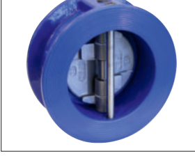
Figure 682 200 PSI CAST IRON WAFER DOUBLE DOOR CHECK VALVE • 200 PSI NON-SHOCK • RESILIENT SEAT • NON-SLAM STAINLESS STEEL SPRING ACTUATED • STAINLESS STEEL DISCS • SIZES 2" - 10"
