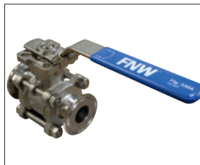
Figure 330A SANITARY 3 PC FULL PORT 400 CWP SS BALL VALVE • CLAMP ENDS • 150 PSI WSP • CAVITY FILLED SEATS • ISO 5211 MOUNTING PAD • SS LOCKING HANDLE • TFM SEATS • SIZES 1/2" - 4"
