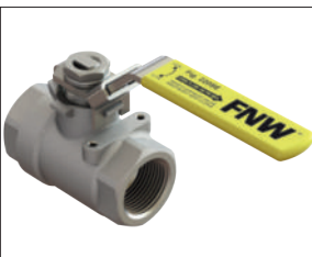
Figure 220SE 2 PC FULL PORT 150 PSI SAFETY EXHAUST BALL VALVE • VENTS DOWNSTREAM PRESSURE IN CLOSED POSITION • INVESTMENT CAST BODY & END CAP • 150 PSI MAXIMUM PRESSURE • NON-VENTED BALL • SS LOCKING HANDLE • RTFE SEATS • SIZES 3/4" - 1 1/2"
