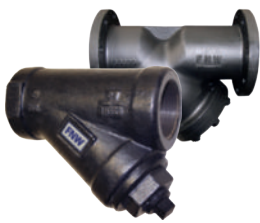
Figure 558A / 559 CAST IRON Y-STRAINER • 125# FLANGED ENDS (558A) & FNPT ENDS (559) • 200 WOG, 125 PSI STEAM (558A) • 400 WOG, 250 PSI STEAM (559) • STAINLESS STEEL SCREEN • SIZES 2" - 12" (558A); SIZES 1/2" - 2 1/2" (559) (2 1/2" IS BOLTED END BONNET)
