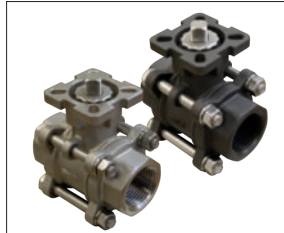
Figure 310AM - SSxSS Figure 311AM - CSxSS 3 PC FULL PORT 1000 CWP ISO MOUNT SS BALL VALVE • ISO 5211 MOUNTING PAD • 150 PSI WSP • LIVE LOADED PACKING • INVESTMENT CAST BODY & END CAPS • NPT ENDS (OPTIONAL SOCKET WELD) • SIZES 1/4" - 4" (4" INCLUDES HANDLE)
