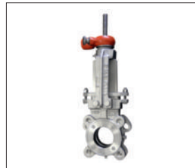
Figure FNW2020TIVTM TRANSMITTER ISOLATION VALVE • CAST SS BODY/YOKE/FOLLOWER • FLEX TEFLON RESILIENT SEATS • BI-DIRECTIONAL SHUTOFF • RATCHET OPERATOR • TANK SIDE FLANGE ACCESS • SIZE 3"
