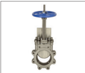
Figure 61B LINED KNIFE GATE VALVE, METAL SEATED • CAST DI BODY/SS LINED • METAL SEAT • SS WETTED PARTS • UNI-DIRECTIONAL SHUTOFF • ECONOMY VALVE FOR MANY APPLICATIONS • SIZES 3" - 24"
