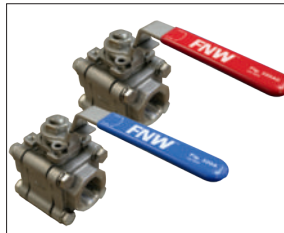
Figure 320A / 320AC - SSxSS Figure 321A / 321AC - CSxSS 3 PC FULL PORT 2000 CWP BALL VALVE • 150 PSI WSP (320A/321A) • 250 PSI WSP (320AC/321AC) • NPT END (OPTIONAL SOCKET WELD) • SS LOCKING HANDLE • TFM SEATS • SIZES 1/4" - 2"
