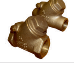
Figure 1241 / 1242 150# Y-PATTERN BRONZE SWING CHECK VALVE • 300 WOG • 150 PSI SATURATED STEAM RATED • RESILIENT SEAT DISC • FNPT (1241) & SWEAT (1242) ENDS • CONFORMS TO MSS SP-80 • SIZES 1/2" - 3"
