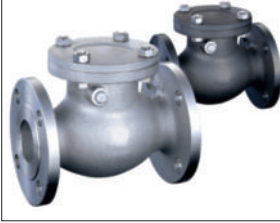
Figure 471A / 472A - SS Figure 571 / 572 - CS FLANGED SWING CHECK VALVE • 150# FLANGES (471A/571) • 300# FLANGES (472A/572) • API 600 (CS), API 603 (SS) • MACHINED DISC & SEAT FOR TIGHT SHUTOFF
