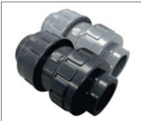
Figure 345 - PVC Figure 355 - CPVC THERMOPLASTIC DOUBLE UNION BALL CHECK VALVE • BOTH NPT & SW ENDS • 150 PSI MAX. WORKING PRESSURE • 5 PSI MINIMUM SHUTOFF • FOR VERTICAL INSTALLATION • EASY MAINTENANCE • SIZES 1/2" - 2"
