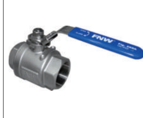
Figure 260A 2 PC FULL PORT STAINLESS STEEL BALL VALVE 1000 WOG • 150 PSI/WSP • WORKING TEMP: -4°F - 392°F • INVESTMENT CAST BODY • BLOW-OUT PROOF STEM • STAINLESS HANDLE • LOCKING LEVER • SIZES 1/4" - 2"
