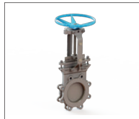
Figure 6800 CAST SS KNIFE GATE VALVE, RESILIENT SEAT • CAST SS BODY/YOKE/FOLLOWER • POSITIVE SHUTOFF RESILIENT SEAT EVEN AT LOW MEDIA PRESSURES • BI-DIRECTIONAL SHUTOFF • STAINLESS NEEDLE BEARING FOR REDUCED HW TORQUE • ANTI-EXTRUSION STRIPS IN PACKING • SIZES 3" - 30"
