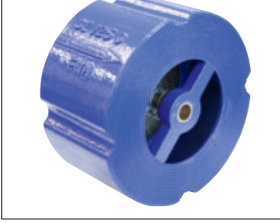
Figure 681 200 PSI CAST IRON WAFER SILENT CHECK VALVE • 200 PSI NON-SHOCK • RESILIENT SEAT • NON-SLAM STAINLESS STEEL SPRING ACTUATED • ALUMINUM-BRONZE DISC • SIZES 2" - 10"
