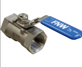
Figure 100A 1 PC STANDARD PORT 1000 CWP STAINLESS STEEL BALL VALVE • INVESTMENT CAST BODY • 150 PSI WSP • SS LOCKING HANDLE • RTFE SEATS • BLOW-OUT PROOF STEM • SIZES 1/4" - 2"
