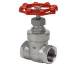
Figure 15B-200 THREADED SS 200 WOG NON-RISING STEM GATE VALVE • STAINLESS STEEL TRIM • ADJUSTABLE PACKING • SIZES 1/2" - 2"
